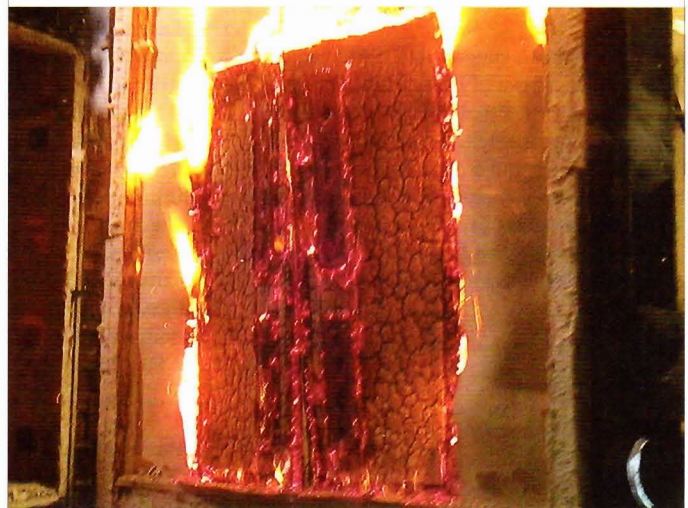
Fire door testing at Exova. The rear of doors after an hour at 1,000°C
