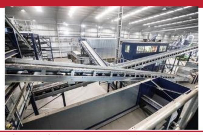
N+P's Teesside fuel preparation plant is designed to receive over 250,000 t per annum of waste paper, cardboard and plastic to produce over 150,000 t per annum of alternative fuel to supply into various industries including, cement, power generation, steel blast furnaces and the lime industry.
