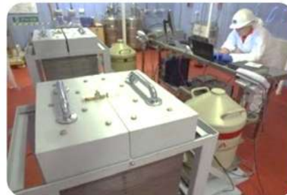
ERSaB: Gamma spectroscopy & low background counting environmental radioactivity studies
