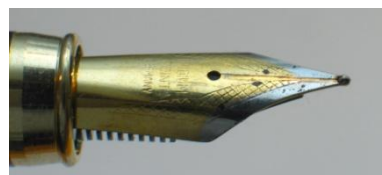
Osmium alloys have been used for the tips of fountain pen nibs From http://en.wikipedia.org/wiki/File:Fountain-pen-nib.jpg
