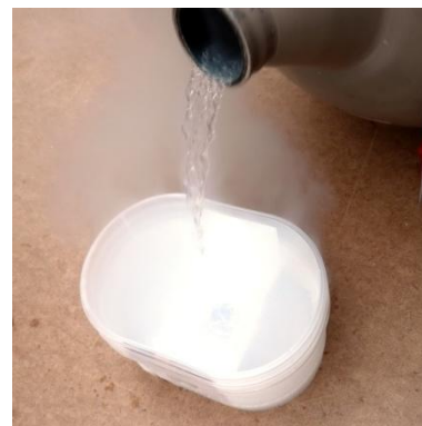
Liquid nitrogen is a colourless liquid which boils at -196^{\circ}\text{C} . From http://en.wikipedia.org/wiki/File:Liquidntr nitrogen.jpg .
