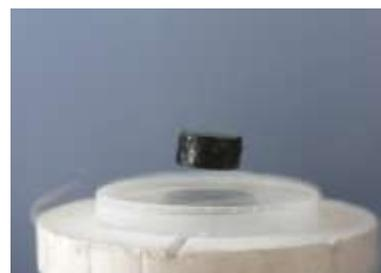
Magnet levitating above a high temperature YBCO superconductor.
