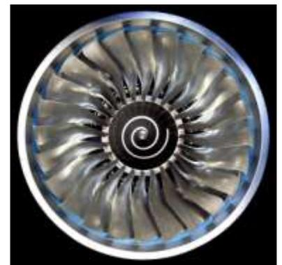
The fan on the Rolls Royce Trent 900 engine is 2.9 metres in diameter.
