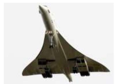
The nose cone and the leading edges of the wings and tail of Concorde had to be made from stainless steel to withstand the temperatures reached through frictional heating.
