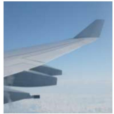
This winglet is fitted to the end of the wing of an Airbus A340-600 aircraft.
