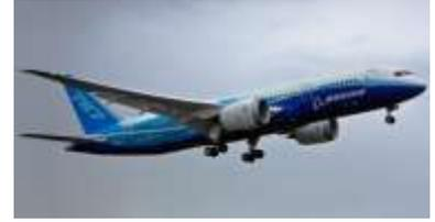
The fuselage of the Boeing 787 is made from carbon fibre epoxy composite.
