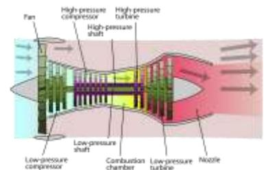
Turbo fan engines work on a simple 4 stage process.
