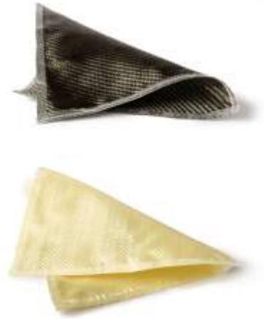
Carbon fibre or Kevlar fibre cloth can be used to make fibre reinforced composites which are light and strong.
