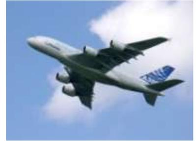
The fuselage of the A380 is made from GLARE and other parts including the vertical tail and fixed trailing edge of the wings are made from carbon fibre composite.
