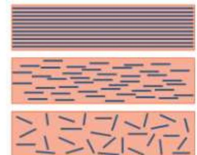
The fibres in a composite may be (a) continuous, (b) discontinuous but aligned, (c) discontinuous and randomly oriented.
