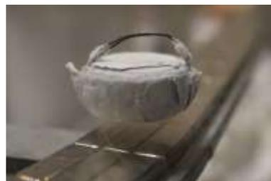
Figure 6 – Superconductor levitating above a magnet. From [http://upload.wikimedia.org/wikipedia/commons/3/3c/Stickstoff\\_gek%C3%BChltler\\_Supraleiter\\_schwebt\\_%C3%BCber\\_Dauermagneten\\_2009-06-21.jpg](http://upload.wikimedia.org/wikipedia/commons/3/3c/Stickstoff_gek%C3%BChltler_Supraleiter_schwebt_%C3%BCber_Dauermagneten_2009-06-21.jpg)
