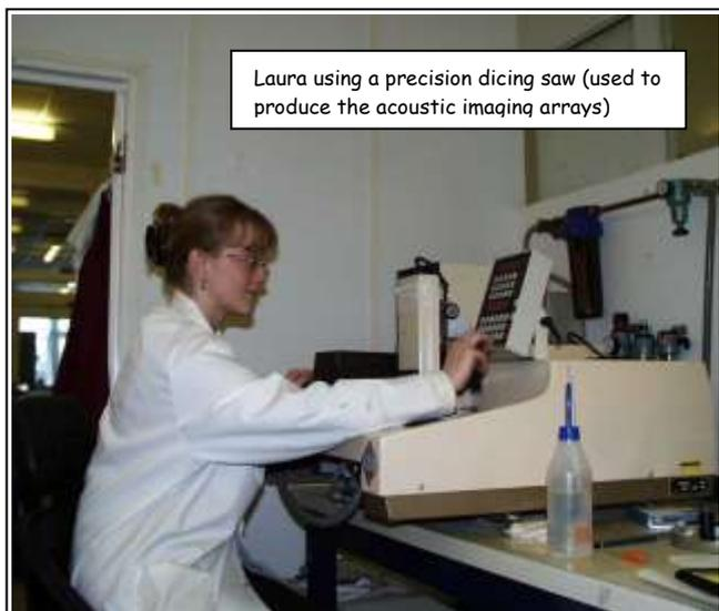
Laura using a precision dicing saw (used to produce the acoustic imaging arrays)
