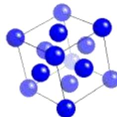
Face centred cubic crystal structure of copper
