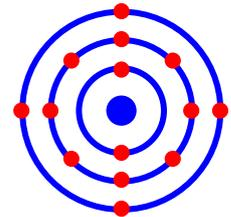
*Electron configuration in a silicon atom showing 4 outer electrons*
