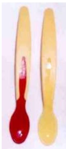
*Thermochromic baby spoon at room temperature (left) and after immersion in boiling water (right)*
