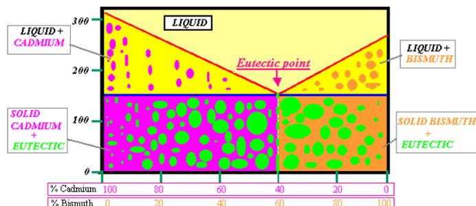
These two metals are completely soluble in the liquid state in all proportions, but become insoluble in the solid state. The Thermal Equilibrium Diagram (TED) or Phase Diagram for this system is shown right. This diagram also shows schematically the phases that are present at different compositions. If an alloy containing 40% cadmium and 60% bismuth by weight is cooled from the liquid state. At 140°C a eutectic structure forms which is made up from alternating
