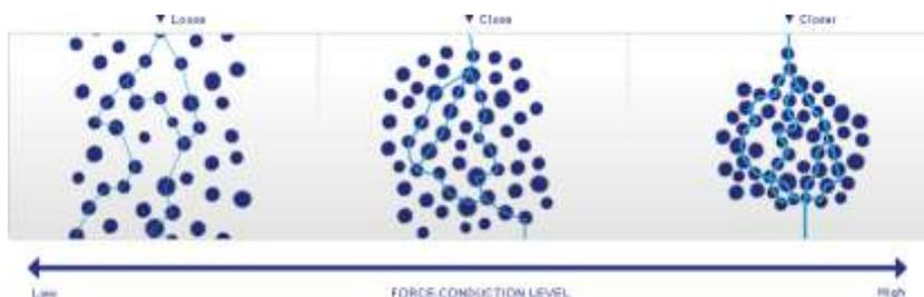
The applied voltage also has an influence on the properties of QTC. At low applied voltages the electrons only have a small amount of energy and cannot tunnel across sizeable gaps between particles in significant numbers. Thus in the unstressed state the material is a near perfect insulator. Applying pressure decreases resistance by reducing the gap between the particles and increasing the probability of tunnelling.
