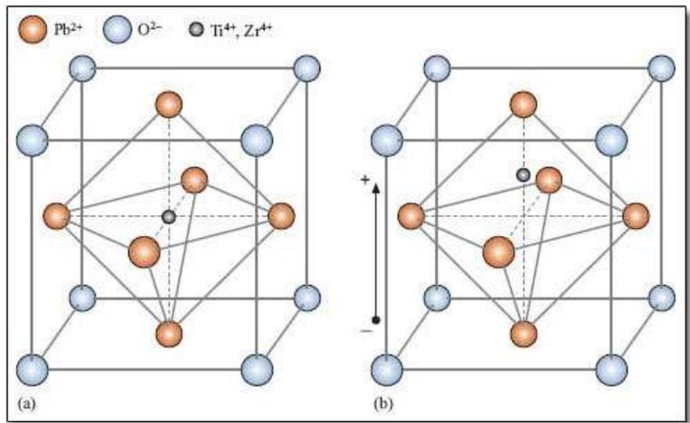
(a) crystal structure of PZT and (b) structure in presence of electrical field showing slight movement of central ion.
