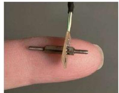
This 10-mm Squiggle motor can be used in mobile-phone autofocus cameras, optical zoom assemblies, and other small products.
