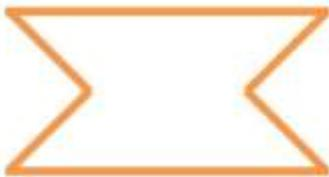
When a tensile force is applied to an auxetic hexagon it experiences extension parallel to the applied force, but also expands perpendicular to the force as the hinge structure unfolds.
