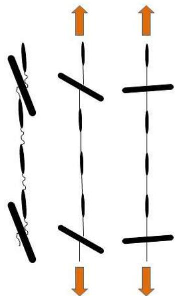
Schematic diagram showing how lateral expansion occurs under tension in a nodule and fibril auxetic material.
