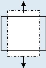
When a compressive load is applied to a cube of material it will tend to contract in the direction parallel to the load (axial direction) and expand in the two directions transverse or perpendicular to the load (see below).
