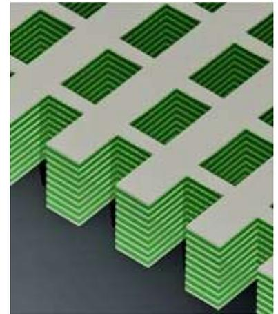
This engineered meta-material has been designed to reverse the direction of visible and near infrared light. It could be used in the development of imaging devices with higher resolution and nanocircuits.
