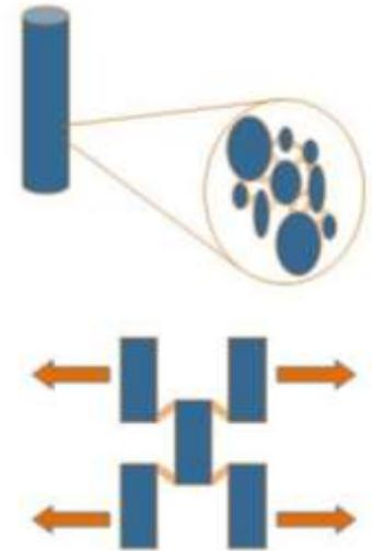
Schematic diagram of nodule and fibril auxetic material (top) showing idealised structure (bottom).
