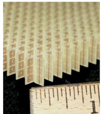
This array has been engineered by mounting an array of split-ring copper resonators on interlocking sheets of fibreglass circuit board. The array is 10x100x100mm in size and consists of three 20x20 unit cells. It has been designed to have a negative refractive index.
