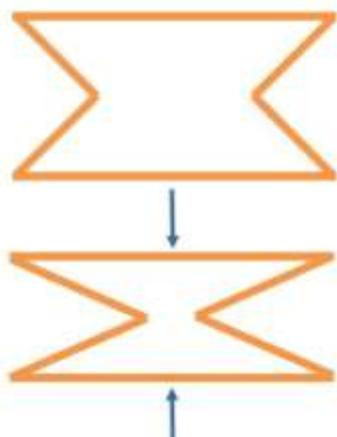
When a compressive force is applied to an auxetic hexagon it experiences a contraction parallel to the applied force, but also contracts perpendicular to the force as the hinge structure folds.
