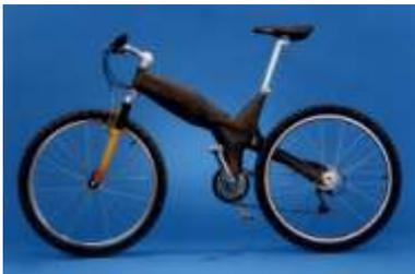
Carbon fibre composite bicycle frame, offering strength, stiffness and low weight.
