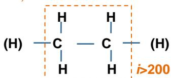
Above a critical number of repeat units neither the end groups nor the chain length affect the properties very much and the resulting materials are known as polyethylenes. Linear polyethylene is a solid, m.p.  $\sim 130^{\circ}\text{C}$ .
