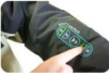
Soft switch built into the sleeve of a jacket uses QTC to control an MP3 player in the wearers inside pocket.
