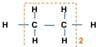
When the molecule consists of two capped repeat units the result is butane gas (m.p.  $-135^{\circ}\text{C}$ , b.p.  $-0.5^{\circ}\text{C}$ ).
