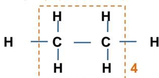
When the molecule consists of four capped repeat units the result is n-octane liquid (m.p.  $-135^{\circ}\text{C}$ , b.p.  $125^{\circ}\text{C}$ )
