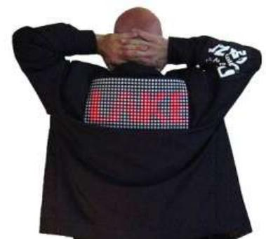
Jacket with integrated digital display consisting of LEDs mounted on to a flexible conducting material.
