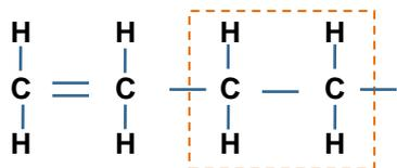
Removal of the double bond from the ethylene monomer (left) produces the ethylene repeat unit or 'mer' (right) which has active sites on each end and is able to form chains
