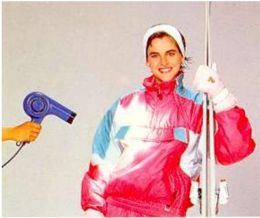
Ski jacket incorporating thermochromic yarn which changes colour when heated.
