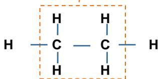
When the molecule consists of one capped 'mer' the result is ethane gas (m.p.  $-172^{\circ}\text{C}$ , b.p.  $-89^{\circ}\text{C}$ ), above.
