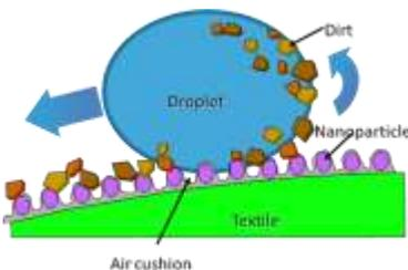
Schematic diagram showing how a nanoscale superhydrophobic coating on fabric repels water and improves stain resistance.
