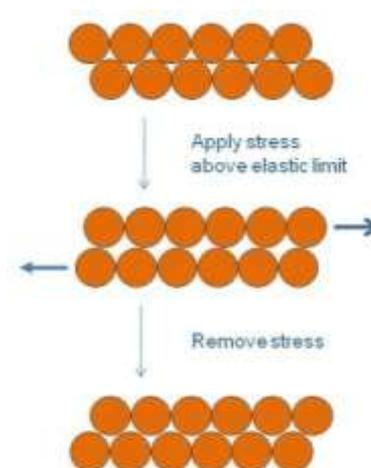
Schematic diagram showing movement of atoms when a stress above the elastic limit is applied
