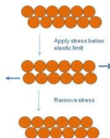
Schematic diagram showing movement of atoms when a stress below the elastic limit is applied
