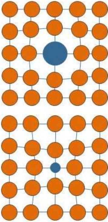
Schematic diagrams showing strain induced in the lattice of a substitutional alloy when the solute atoms are larger (top) and smaller (bottom) than the solvent atoms.
