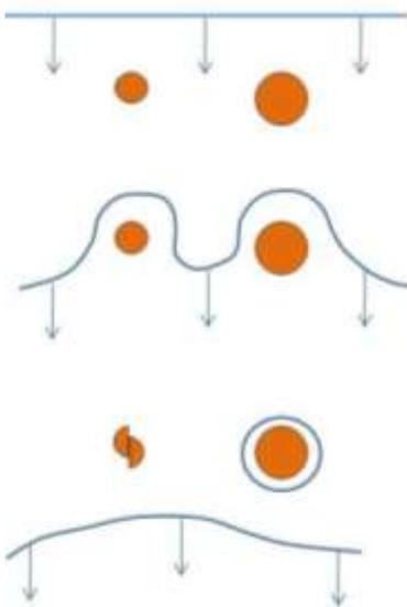
Schematic diagram showing the interaction of a moving dislocation (blue) with a small particle and a large particle. The dislocation cuts through the small particle but loops around the large one.
