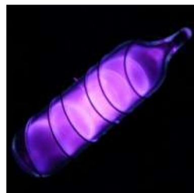
Characteristic purple glow of argon gas placed in a high voltage electric field.
