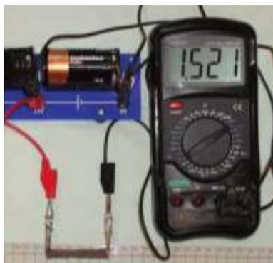
Photo 2 – Potential difference across the battery when strip is connected.
