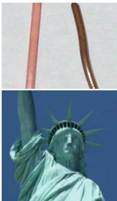
Figure 5 – Pure copper takes on a peachy colour (top left), but this soon dulls on expose to air as a black oxide layer forms (top right). If corrosion is allowed to continue the green-coloured patina known as verdigris forms. This gives the Statue of Liberty her characteristic colour.
