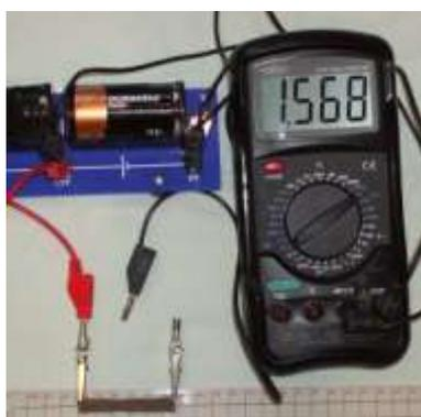
Photo 3 – Potential difference across the battery in open circuit.
