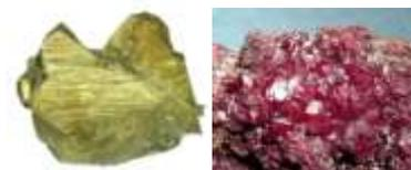
Figure 7 – Copper containing minerals chalcopyrite,  $\text{CuFeS}_2$  (left) and cuprite  $\text{Cu}_2\text{O}$  (Right).
