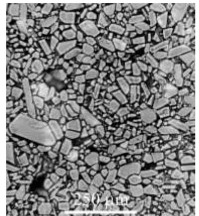
Figure 5 – Microstructure of an alumina ceramic composed of 96% Al<sub>2</sub>O<sub>3</sub>, with the remainder a mixture of MgO, CaO and SiO<sub>2</sub>. The light coloured phase is angular particles of alumina and the dark coloured matrix is an aluminosilicate glass. (<http://www.doitpoms.ac.uk/miclib/micrograph.php?id=198>)
