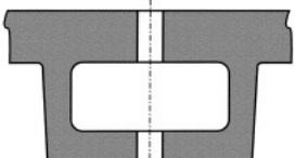
**Preferred design.** Coring of the boss will maintain the uniformity of casting cross section, reducing the risk of porosity in the casting and under-firing.
