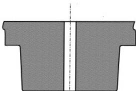
**Poor design.** The large change in cross section of this boss will cause problems with porosity in the casting, and with localised under-firing of the vitreous enamel.
