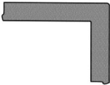
**Poor design.** The corner is too sharp. The enamel will tend to burn off the corner during firing and even if a full coat can be achieved it will be very susceptible to chipping. It will be very difficult to coat the sharp corner to achieve a full coat of vitreous enamel.
