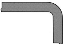
**Preferred design.** The radiused corner will be easier to coat with vitreous enamel, will be much less susceptible to chipping and less prone to burn off during firing. All radii on the casting which will be coated need to be similarly generously radiused.
