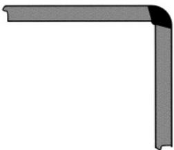
**Poor design.** The weld has been made along an edge. As well as the difficulty of producing a sound weld in this area, there will be a tendency for stress build up. Even with good dressing the resultant radius is too small and there will be a risk of chipping.
