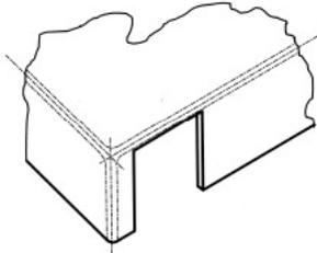
**Poor design.** The large cut out from the flange will result in weakening of the part and will lead to distortion during firing. The design is further aggravated by the sharp corners.
