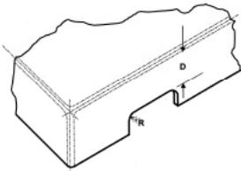
**Preferred design.** The cut out has been minimised retaining strength in the flange by maximising dimension D and the corners have been rounded with a generous radius R.
