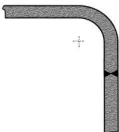
**Preferred design.** Ideally the weld should be placed away from the corner. This permits a suitably generous radius on the edge. In some components, this may not be possible in fully fabricated parts and if so careful and neat after dressing of the weld is critical to the final appearance. The extent of such welds should be kept to a minimum.
