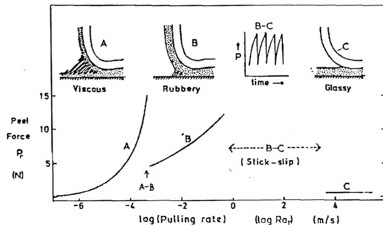
Figure 2 : Dependence of peel force on (log) pulling rate at 296 K for polyester backing/polybutyl acrylate adhesive/glass substrate. Tape is 2.54 cm wide, and other dimensions as shown in figure 1. Drawings illustrate the adhesive behaviour in each region.
