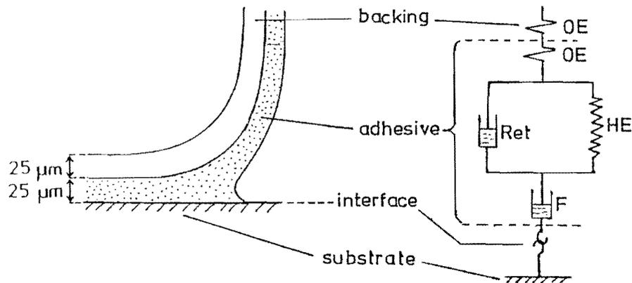
Figure 1 : Peeling joint and assumed mechanical analogue.
