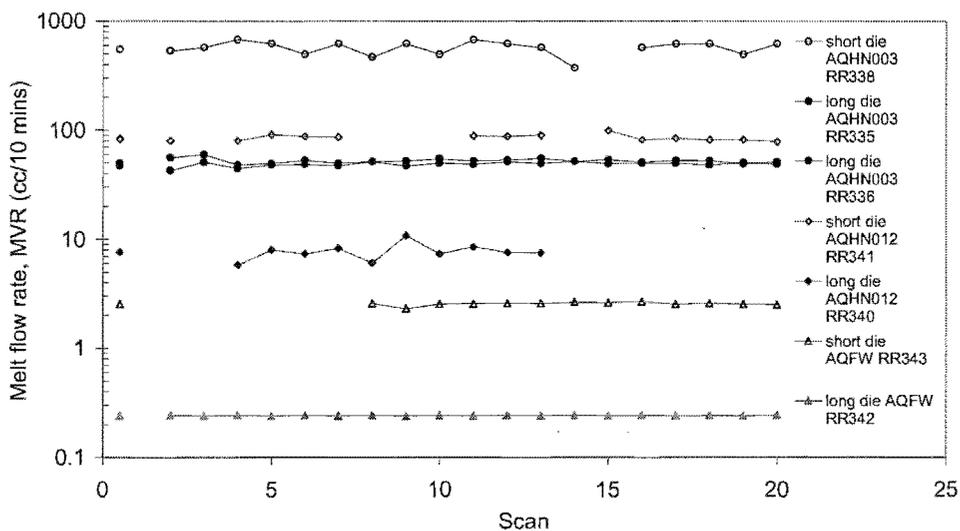
Figure 3: Melt flow rate measurements of three hot melt adhesives using short and long dies, permitting derivation of shear and extensional flow properties.
