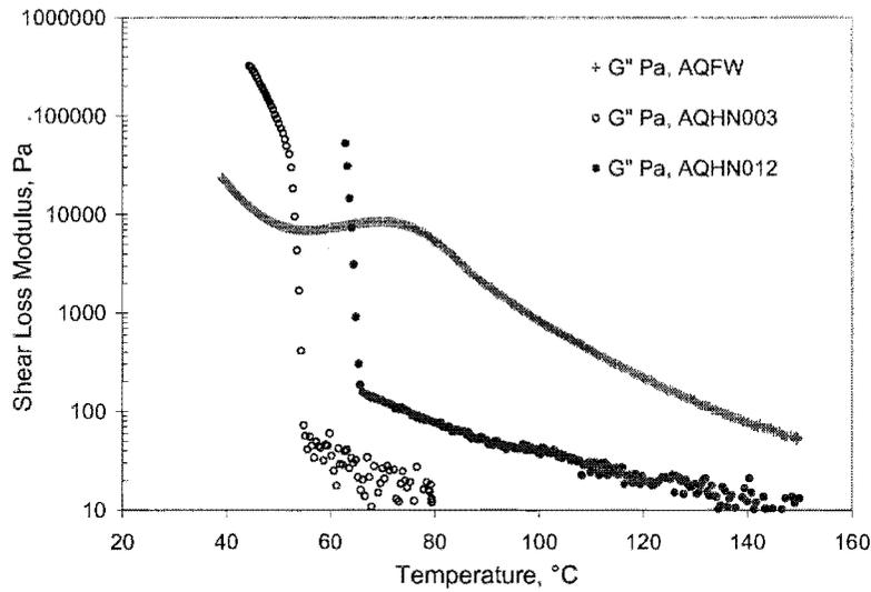
Figure 1: Temperature dependence of hot melt adhesives by oscillatory rheometry, exhibiting significant differences in viscous response. (Material names given are NPL sample codes)
