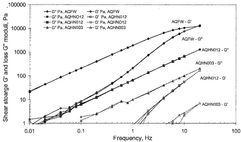
Figure 2: Comparison of the viscoelastic responses of various hot melt adhesives, by oscillatory rheometry.
