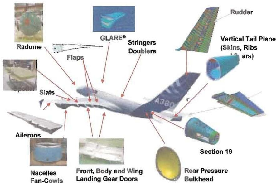
Adhesive bonding offers many advantages to aircraft structures, particularly:
