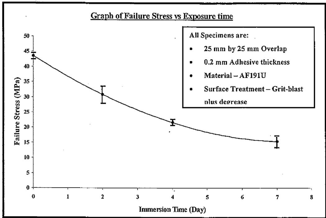
**Figure 2** Effect of water on the strength of single lap joints at various immersion times
