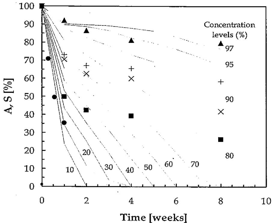
**Figure 4** Proportion of the joint area (A) which is below a given water concentration level after a given time of exposure.
