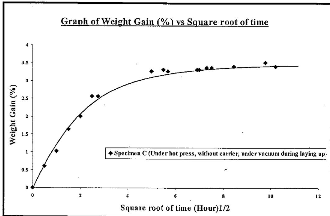
**Figure 1** Water uptake curve for specimen C from the immersion experiment at 70°C
