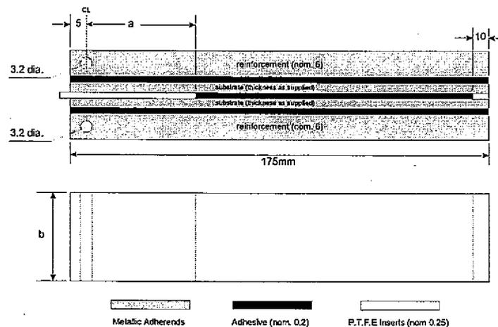
Figure 1 The RDCB test piece used for fatigue testing
