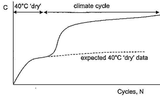
Figure 2 Schematic showing the applied methodology of the RDCB fatigue test
