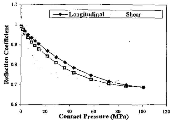
Figure 4. Comparison of shear and longitudinal loading tests.
