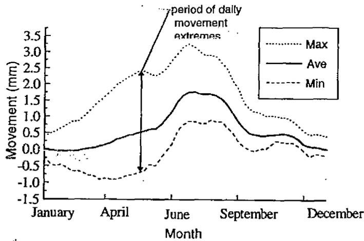
Figure 4. Annual pattern of joint movement for aluminium-clad building
