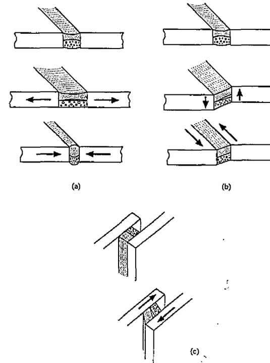
(a) Butt joint in tension/compression; (b) butt joint in shear; (c) lap joint in shear
