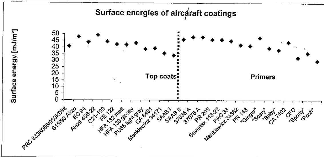
Figure 1: Surface Energies of some Aircraft Coatings
