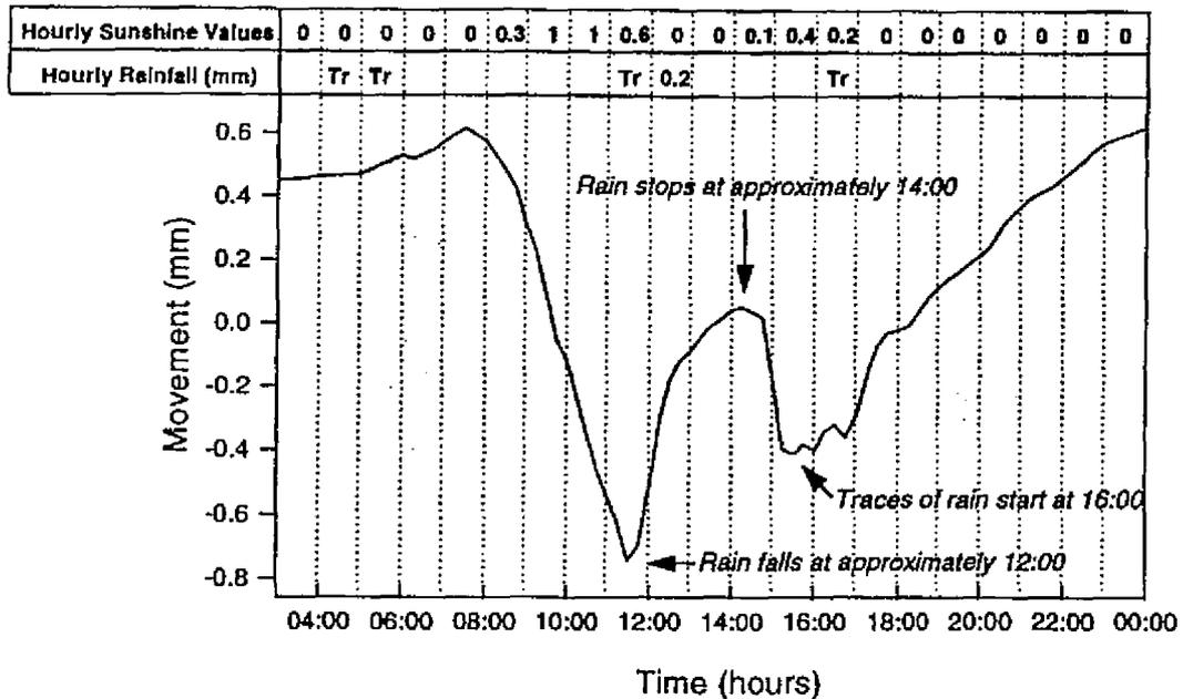
Figure 5. Daily pattern of movement for aluminium-clad panel joint
