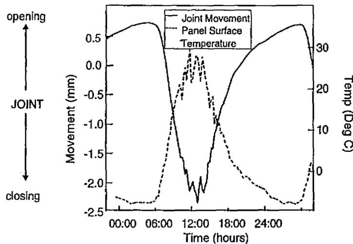
Figure 3. Springtime temperature and movement for aluminium cladding
