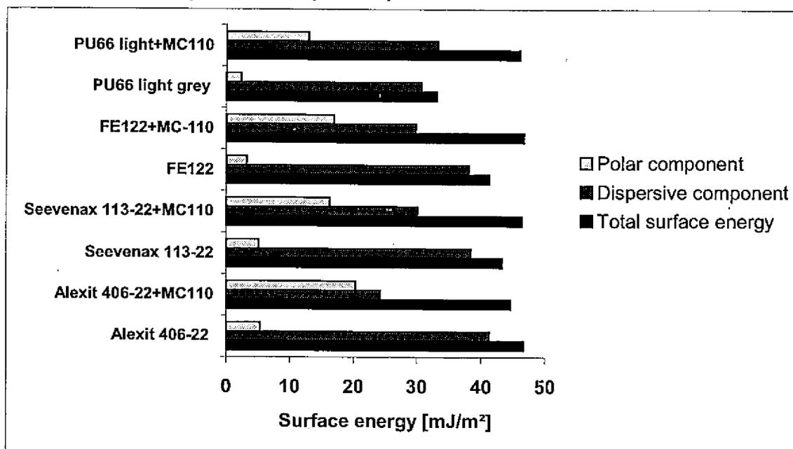
Figure 2: Components of the Total Surface Energy according to Owens-Wendt
