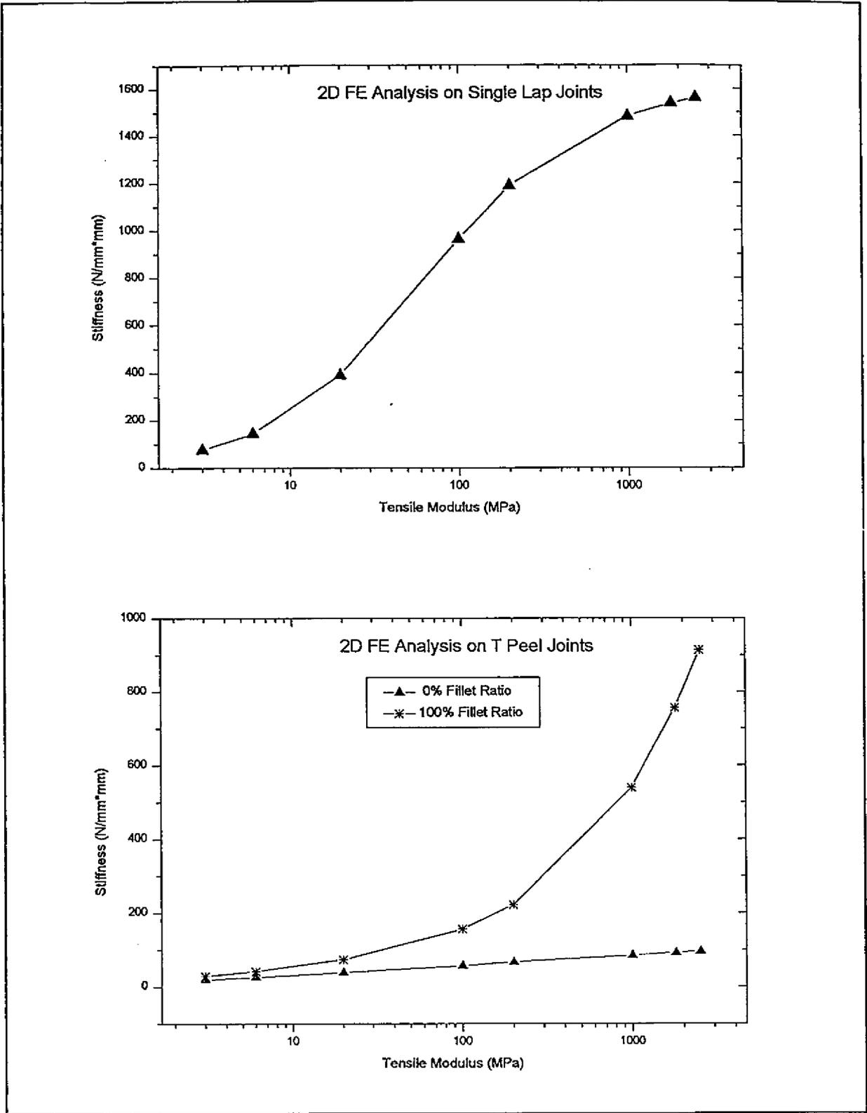
**Figure 2 Effect of adhesive modulus on joint stiffness**
