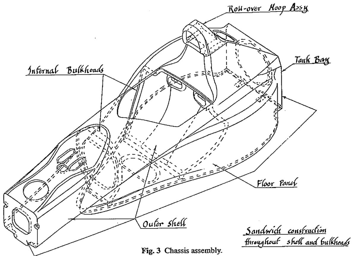
Fig. 3 Chassis assembly.
