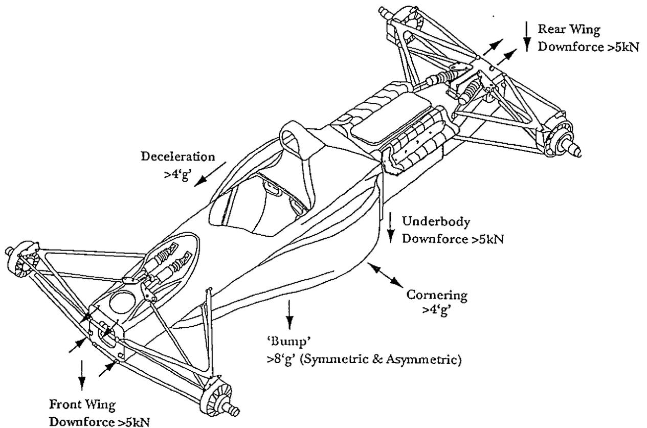
Fig. 4 Chassis inertial load cases.
