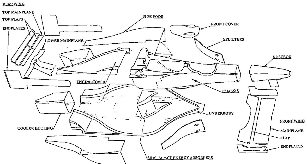
Fig. 2 Components manufactured from composite materials.
