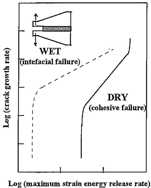
**Figure 2** Schematic of the influence of moisture ingress on the relationship between the rate of crack growth in fatigue and the fracture energy.
