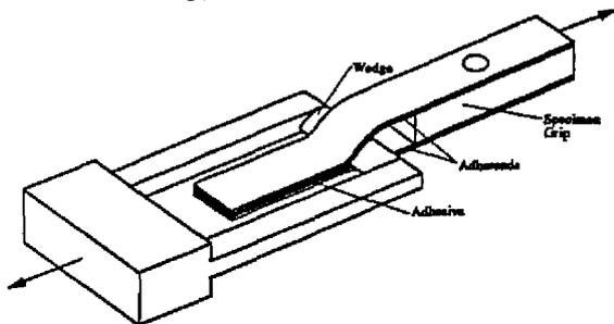
Figure 3: The impact wedge peel (IWP) test.
