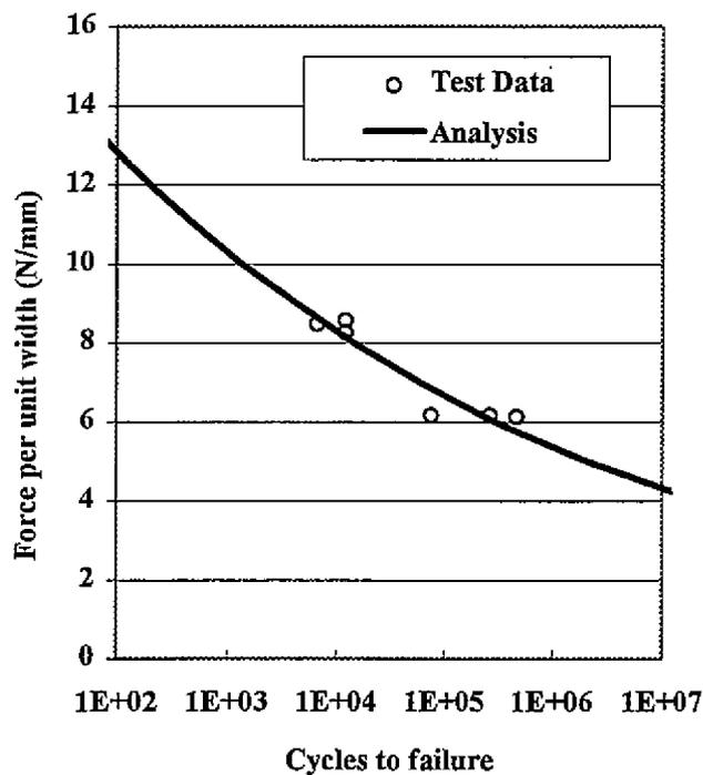
**Figure 4** Assessment of the fatigue life of a structural joint under 'dry' conditions.
