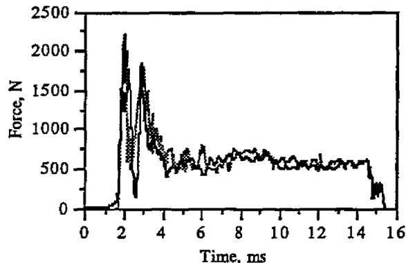
Figure 4: Force versus time trace for steel IWP specimen bonded with XB5315, tested at 2 m/s. Solid line is experimental data, dashed line is FE prediction.
