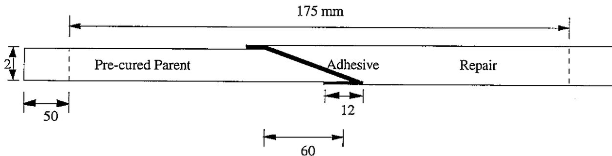
Figure 1: Repair specimen geometry
