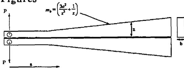
Figure 1: The tapered double cantilever beam (TDCB) test specimen.
