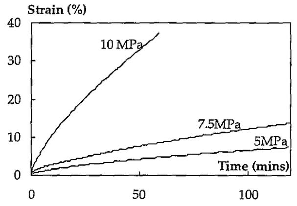
Fig 2 - Creep compliance for adhesive B
