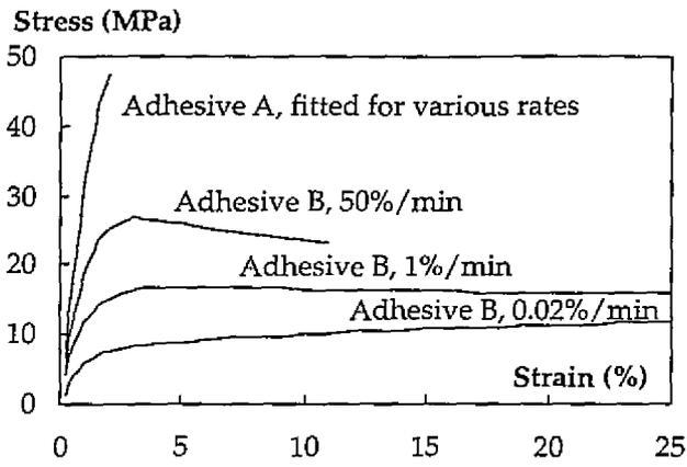
Fig 1 - Stress-strain data for adhesives A and B
