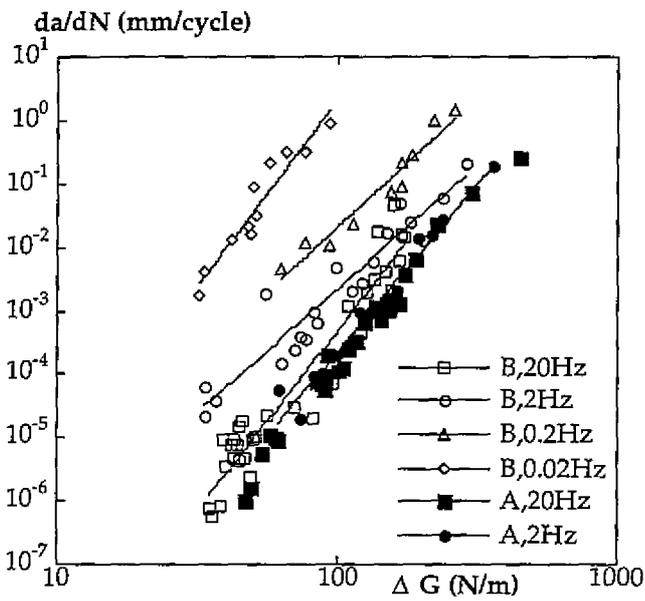
Fig 3 - Cyclic FCGR for DCBs of both adhesives
