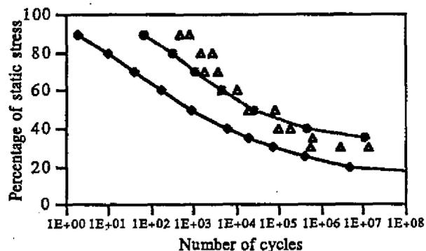
Figure 7: Single lap joints, lifetime prediction: ( $\Delta$ ) experimental, ( $\diamond$ ) theory - analytical, ( $\bullet$ ) theory - finite element. 'AV119' adhesive, steel substrates.
