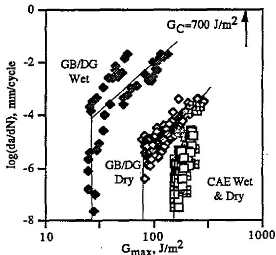
Figure 6: TDCB durability results for 'AV119' adhesive, aluminium alloy adherends.
