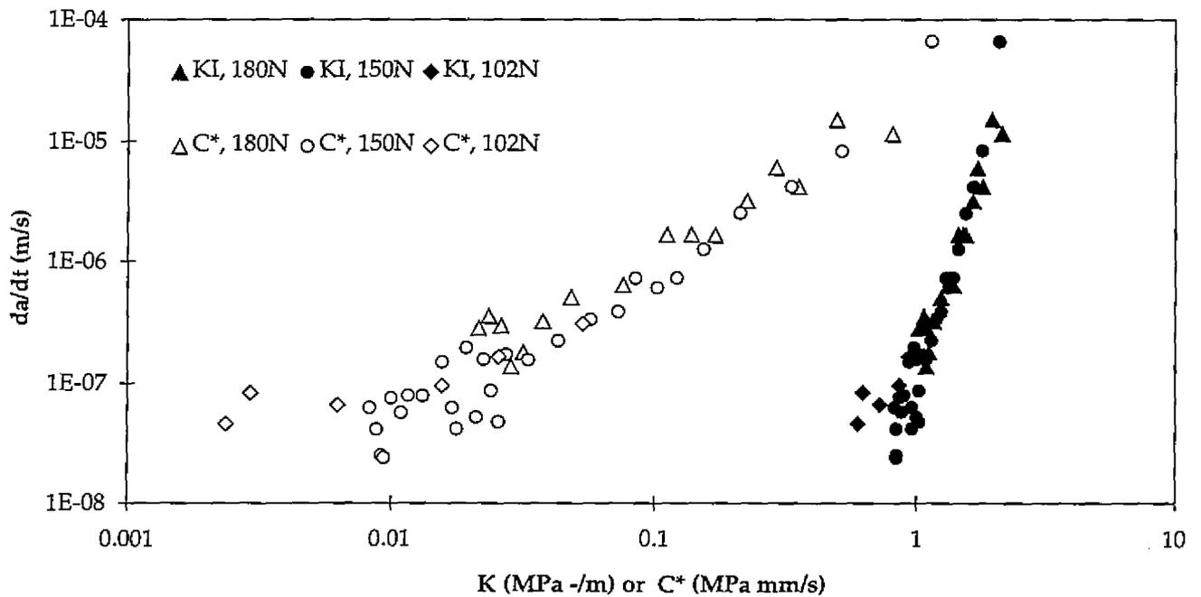
Fig 5 - Creep CGR in bulk CT specimens plotted against LEFM and power law creep parameters
