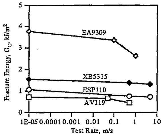
Figure 2: The effect of test rate on adhesive fracture energy, TDCB tests.
