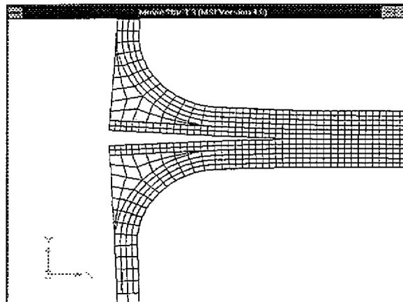
**Figure 3** Deformed mesh from FEA of structural joint with a cohesive crack in the adhesive layer.
