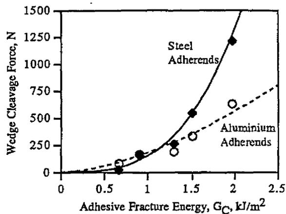
Figure 5: IWP wedge cleavage force versus TDCB fracture energy correlation.
