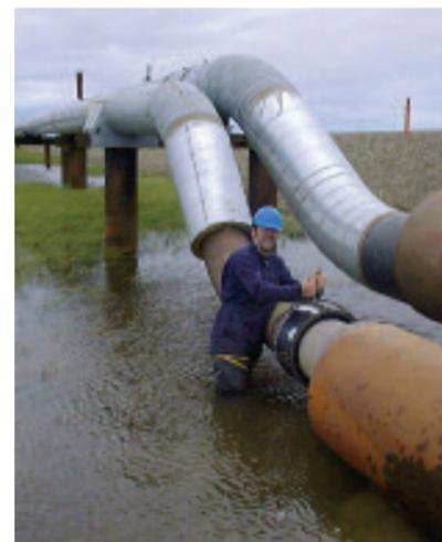
In-service inspection of insulated pipelines using guided wave ultrasonics (Teletest™) (Courtesy: TWI)
