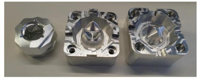
CNC machined inserts (left), female mould (centre), male mould (right).
