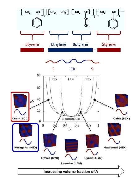
Depending on styrene content and molecular weights, phase separation induces various morphologies:
