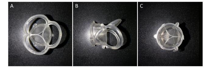
Top view (A), side view (B) and bottom view (C) of injection moulded transcatheter PHV
