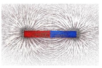
The parts of the magnet where the force lines are closest together and the magnetic field is the strongest are called a **poles**. We call the poles **north** and **south**.
