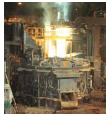
Figure 5 – Electric arc furnace for secondary steelmaking. ( www.scienceinpublic.com )
