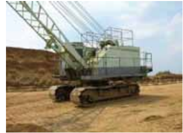
Figure 7 - Typical dragline excavator used to extract sand and gravel.
