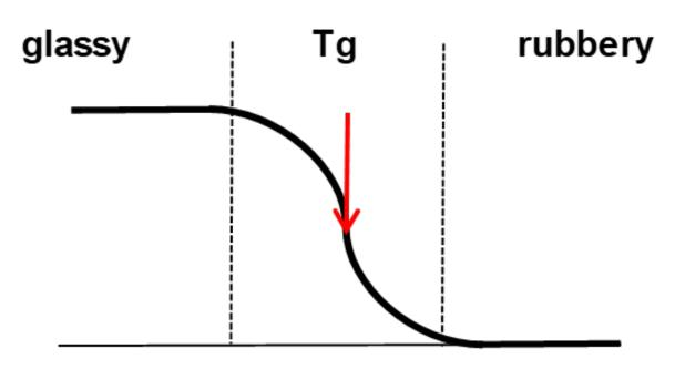
Glass Transition (Tg) is the temperature in which a polymer changes from being elastomeric to being ridged
