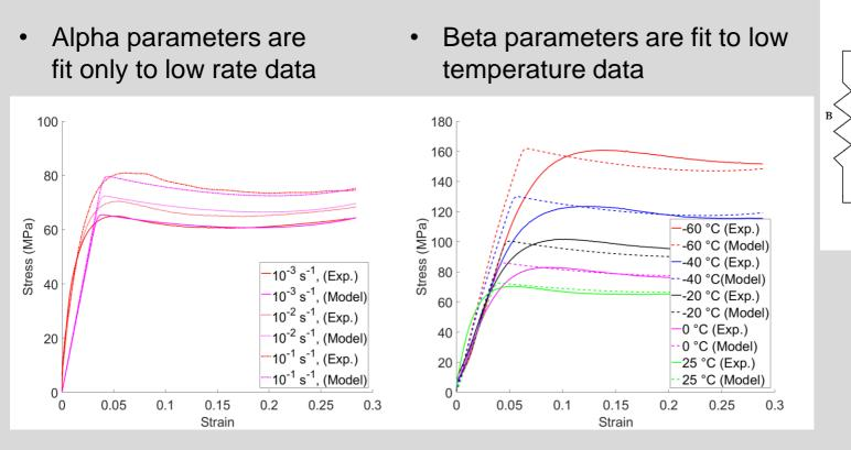
Time-Temperature Superposition principle is key to this approach
