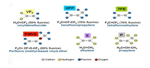
The PMVE is the monomer responsible for the improved low temperature performance of the FKM and this can be replaced with the novel monomer technology which improves this performance without compromising the fluorine content and therefore the chemical resistance.
