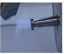
Graphene nanoplatelets are uniformly mixed by ultrasonic vibrations during spray
