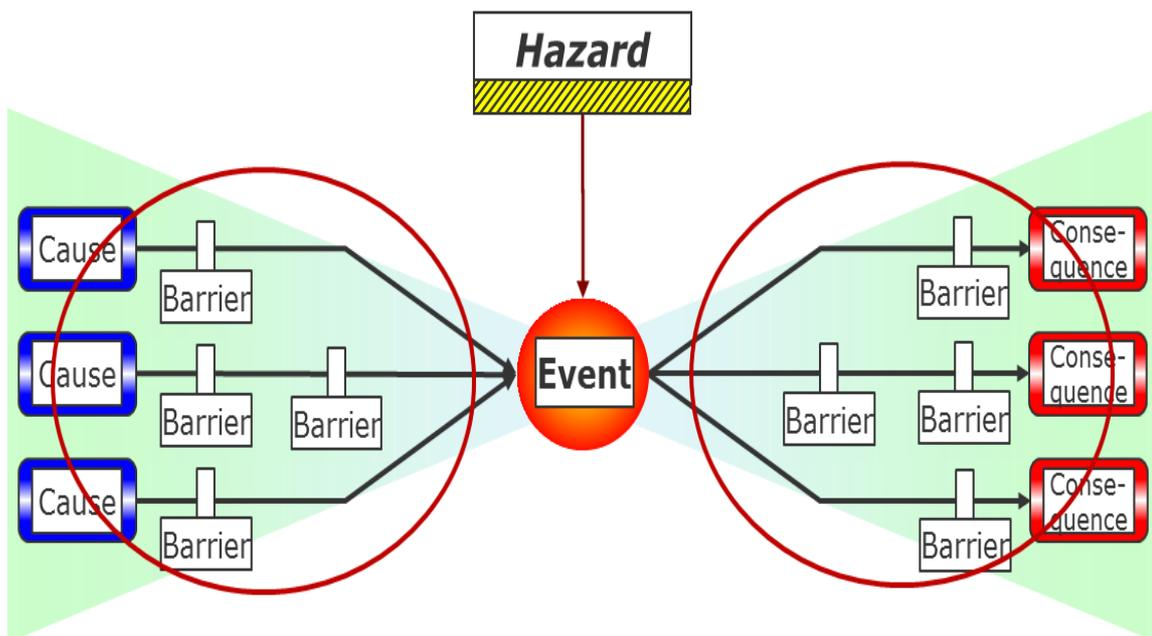
Degradation factors, which weaken the barriers, may also be presented on the bowtie diagram, along with controls that are in place to maintain the effectiveness of a barrier.
