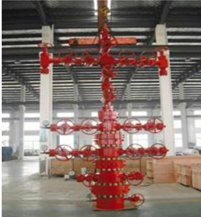
Typically the wellhead will sit below ground level and the surface equipment will be screened from view by trees. The drilling rig will be on the well site for the drilling and completion of the well and will then be moved. Once the Xmas tree has been installed the well will be commissioned or connected to the production facilities.
